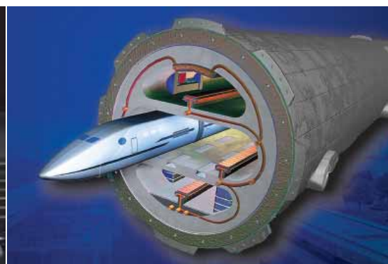
Maglev trains today, like the Japanese MLX01 ( left ) have achieved travel speeds of 581 km/h. In a vacuum tube ( right ), since there is no resistance from the air, maglev trains could reach speeds in excess of 6,000km/h.
