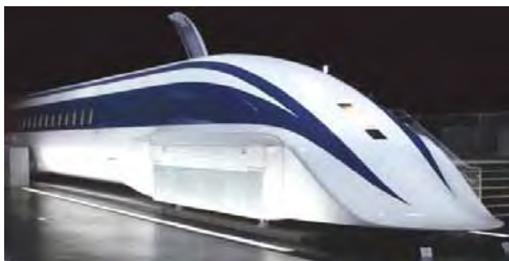
Maglev trains today, like the Japanese MLX01 ( left ) have achieved travel speeds of 581 km/h. In a vacuum tube ( right ), since there is no resistance from the air, maglev trains could reach speeds in excess of 6,000km/h.
