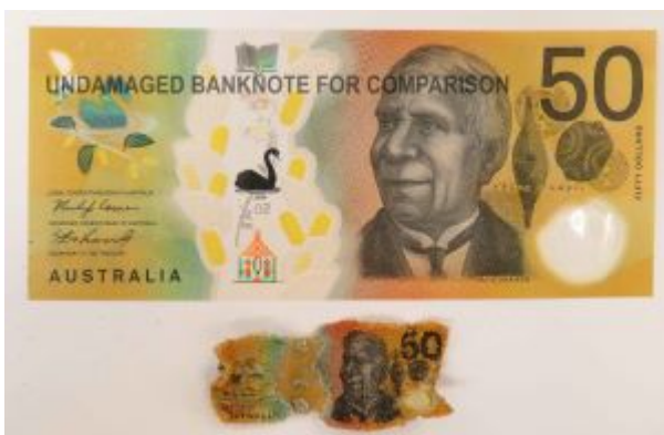
(c) Comparison of a shrunken NGB $50 banknote to its original size
