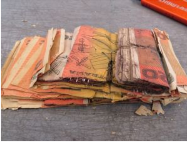
(a) Paper decimal series banknotes that disintegrated from moisture
