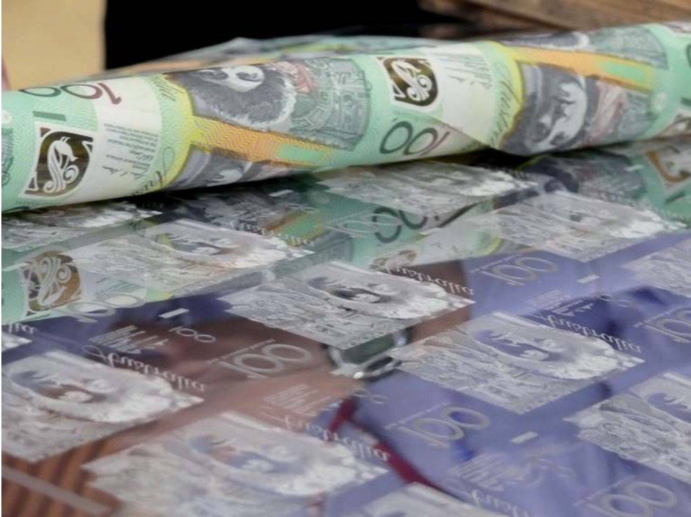
Comparing a printed sheet to an intaglio plate in preparation for a forthcoming $100 note production run.
