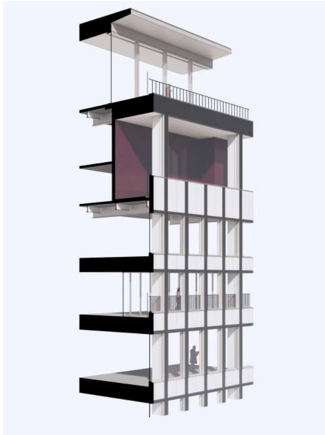
Figure 22 - Indicative section through upper levels 15 through 20 and the roof top pavilion of the building. The plum-coloured glazed tiles to the outside of the original plant rooms will be conserved. (Source: Architectus)
