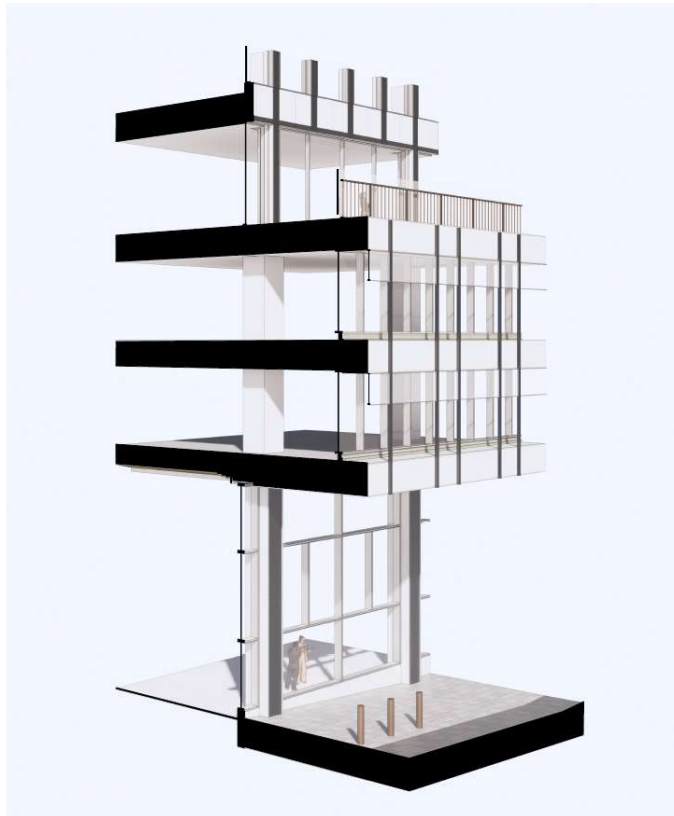
Figure 25 - Section demonstrating the articulation between the podium, the ground level and tower portions of the building. (Source: Architectus)
