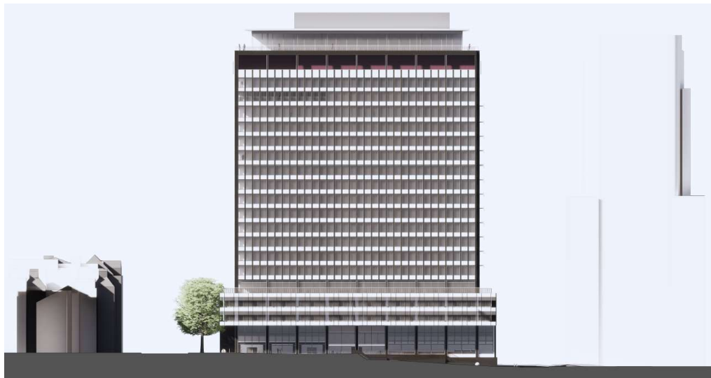
Figure 21 – Diagram of the northern facade, illustrating the relationship between the entry level, the podium and the tower components. Also shown is the 'tartan' pattern applied across the tower facade, and the relationship of the lift over run and rooftop pavilion. (Source: Architectus)
